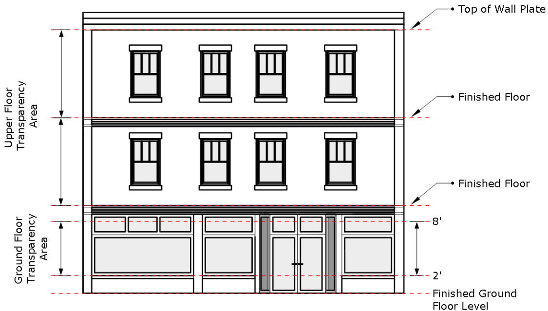
Figure 1315.J: Ground and Upper Floor Transparency Area
