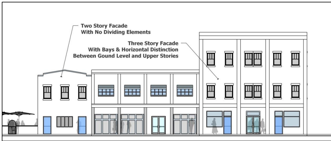
Figure 1327.H: An example of facades of different heights. The two story façade on the left requires no horizontal separation. The three story façade on the right has a horizontal band creating distinction between the ground level and upper floors.
