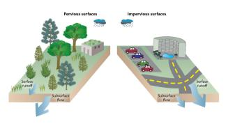
WV's Stormwater General Permit requires new and re-development to reduce the volume of stormwater runoff from development. This is accomplished by mimicking natural, or pre-development hydrology.
